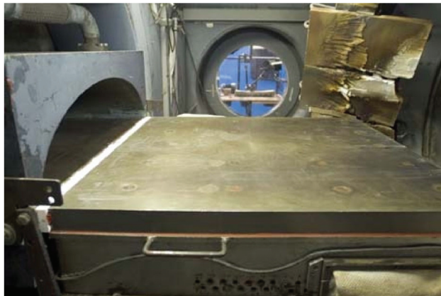
Fig. 2 A photograph of the water-cooled calibration plate flush mounted to the bottom surface of the nozzle and heat flux gage and pressure transducer locations on the 180 deg-rotated plate.
